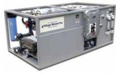
Optional modular configuration allows freedom to install components where space permits, and the modules are small enough to fit through hatchways for installation.
