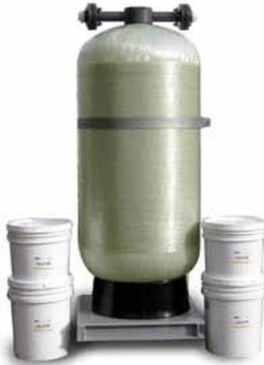
The Racor Village Marine Tec. Remineralizer Systems offer pH neutralization of RO water and are specifically engineered to operate with Village Marine PW and SW Series Watermakers. The media restores a buffer capacity to raise pH and reduce fresh water “aggressiveness” against metal pipes and fixtures. (See bulletin no. 7903)
