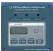
Operate and monitor all of the major functions of your watermaker from the comfort of a bridge or salon. No more trips to the engine room to turn valves or push buttons. The Village Marine Remote Control uses a true pressure regulator that can actually start and stop the system.
